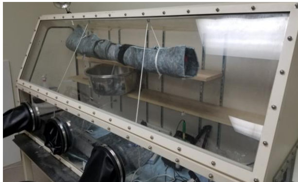
Figure 7. Sediment core handling for the porewater measurement of the inorganic COCs.
