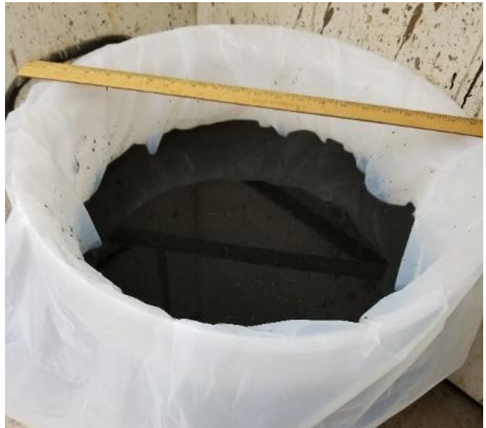
Figure 2. Sediment and water mixture to prepare synthesized porewater.
