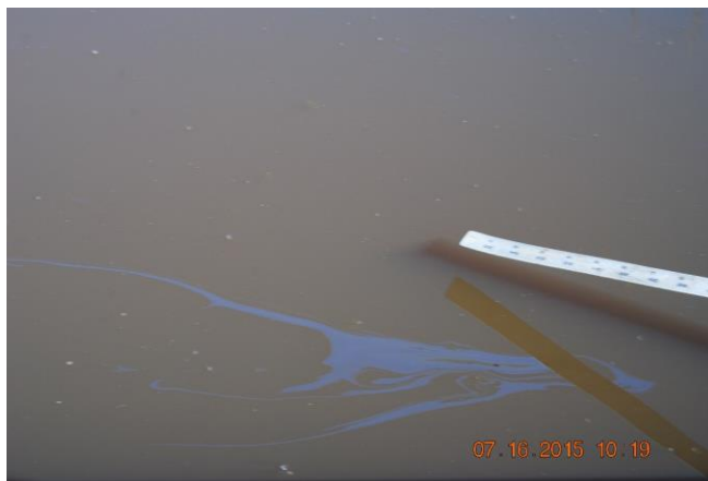
Typical crude oil-related sheen patch/streamer observed at the site.
